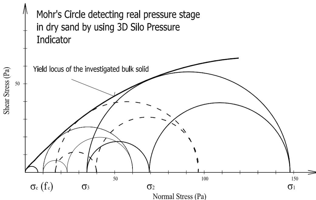
Figure 8 – Shear stresses (in Pascals) Vs. detected normal stresses (in Pascals) on the steel face of the 3D indicator model
