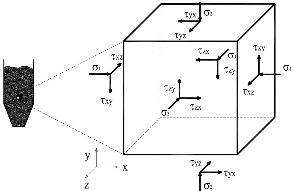
Figure 1 – A small cube (right) takes out of the silo (left) and its rearrangement to principal stress directions for explanation of normal and shear stresses acting on individual cube surfaces
