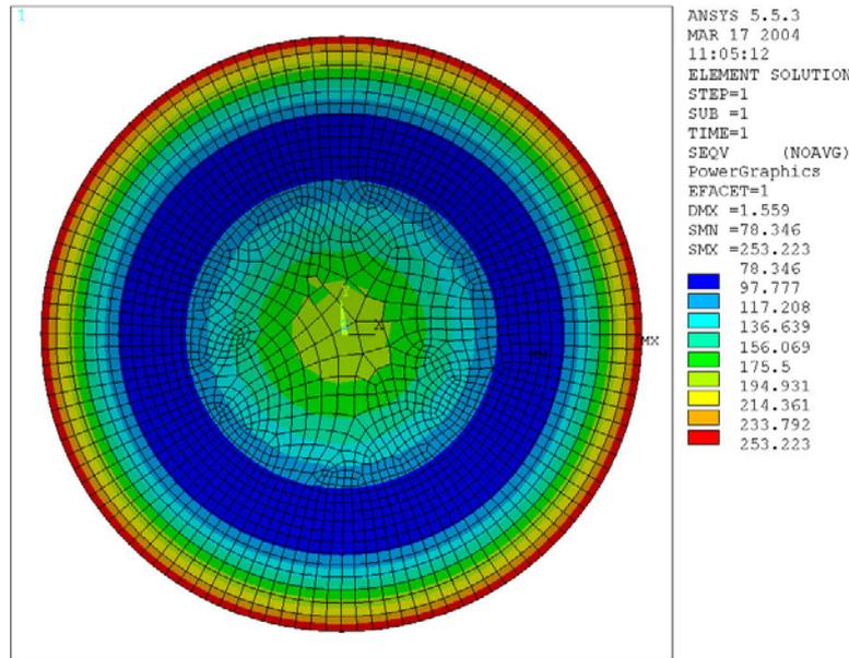
Figure 5 – Stress distribution modelling (in Pascals) on the circle steel face of the 3D indicator model which a detector in the centre is placed on
