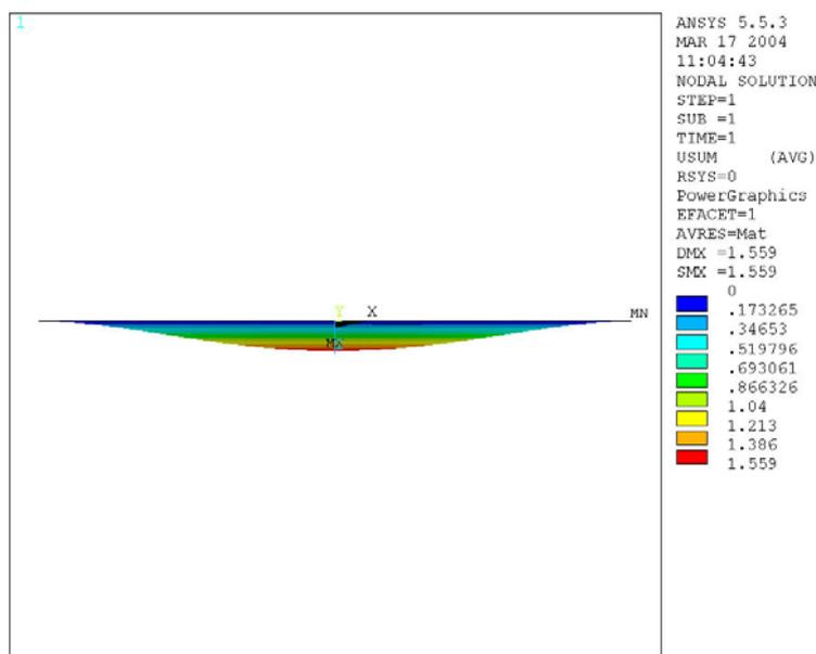
Figure 6 – Deformation distribution modelling (in millimetres) on the circle steel face of the 3D Indicator model which a detector in the centre is placed on
