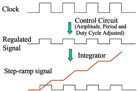
Figure 3 A step-ramp signal.
