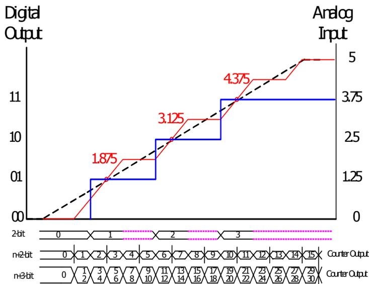
Figure 4 Step-ramp signal mapped to 5-bit counter for 2-bit ADCs.
