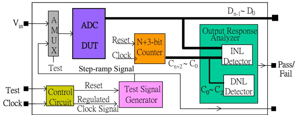
Figure 5 The configuration of BIST structure.
