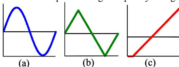
Figure 2 Continuous test signals: (a) sine wave; (b) Triangular wave; (c) rising ramp.
