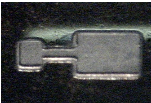
FIGURE 11 Pictures of two different LIGA-like micro accelerometer during microfabrication.
