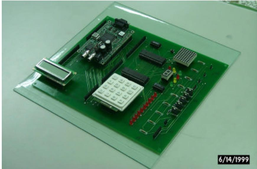
Fig.2 C50 DSK extension board layout
