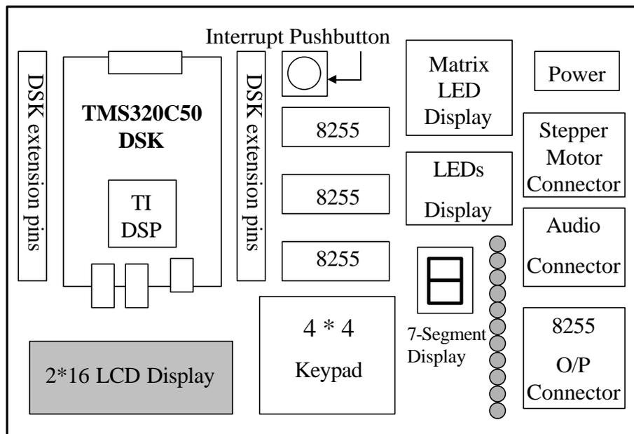
Fig.1 DSK50 Extension Board
