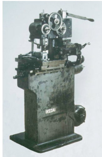
Photo 3. Profile copy reduction shaping machine under reproduction.
