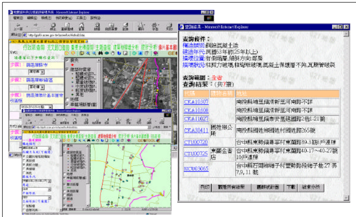
Figure 5 The Thematic Map Overlay and Building Damage Analyses Functions Provided by the Reconnaissance Database Management and Analysis System
