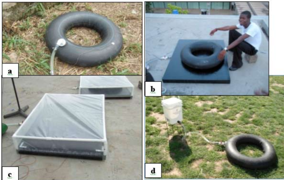
Figure 1. Design – I – Different test configurations. (a) directly on the ground without a cover, (b) insulated from the ground without a cover, (c) insulated from the ground with a cover, and the final design.
