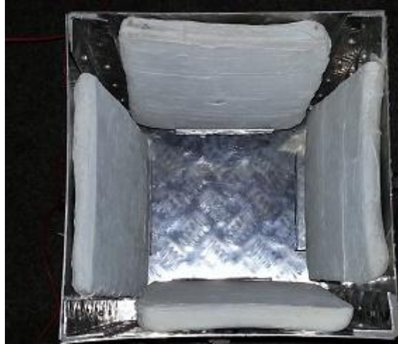
Figure 5: Top view of assembled infrared gasifier
