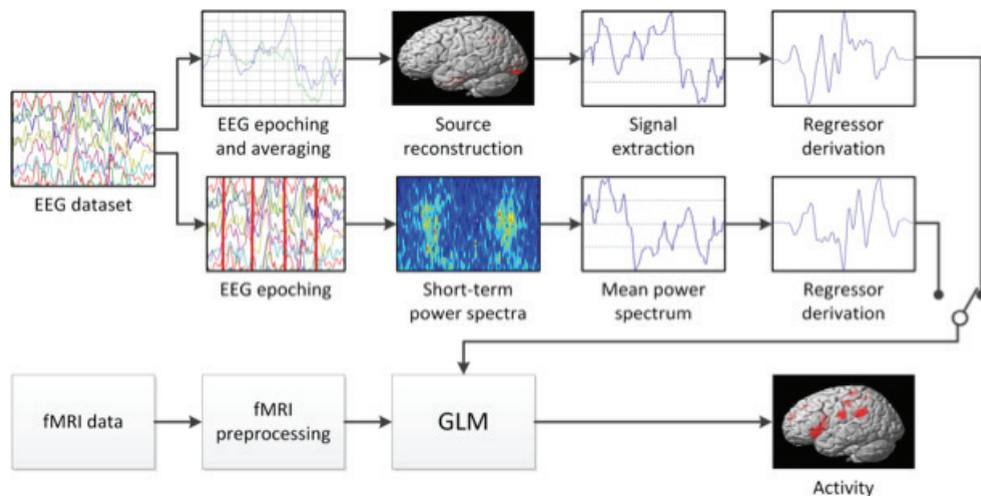
**FIGURE 1.** Flowchart of the proposed techniques of the analysis.
