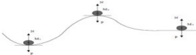
**FIGURE 1.** *Spherical masses in static equilibrium.*
