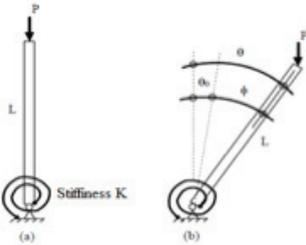
**FIGURE 2.** System showing a no weight rigid bar with imperfections and circular spring.
