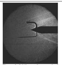
Figure 3: Schlieren photograph of total and static pressure probes in Trisonic Wind Tunnel.
