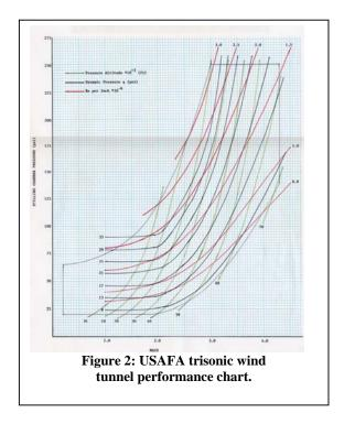
The TWT was originally designed as a force and moment tunnel, and it still functions well in that mode. Over the years other test requirements have led to using the TWT for a variety of tests, including: transverse jet blowing, surface pressure distributions, internal flow, and other diverse testing applications.
