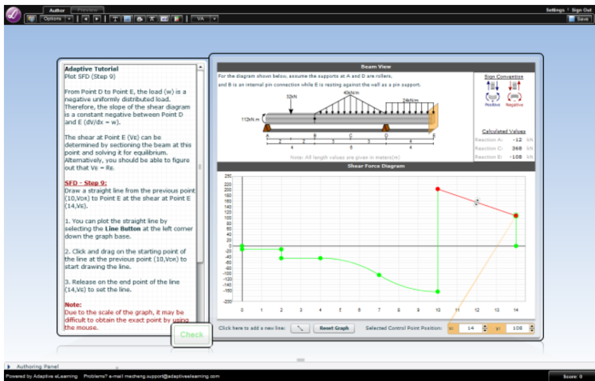
Figure 2: Adaptive tutorial on shear force and bending moment
