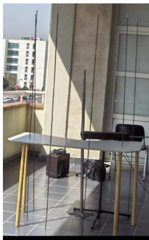
FIGURE 6 ARRAY OF MONOPOLES FOR ISOLATION OF THE THEREMIN PITCH ANTENNA
