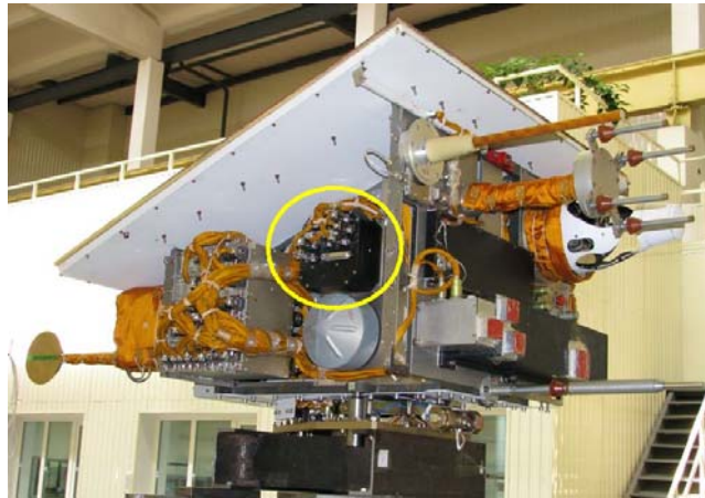
FIGURE 5 ESEMS IN FACTORY. THE YELLOW CIRCLE INDICATES THE LOCATION OF CKB
