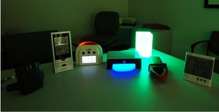
Figure 1. In-home energy displays from left to right: PCM, Aztech, Wattson, Ambient Orb, and Cent-A-Meter
