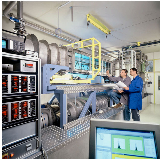
FIGURE 2 MATCHED-INDEX-OF-REFRACTION TUNNEL AT UNI. ERLANGEN
