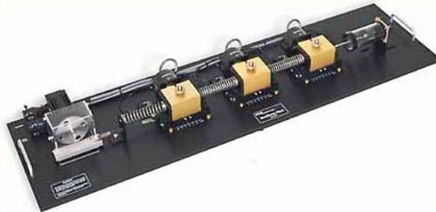
FIGURE 1 ECP 210 RECTILINEAR PLANT AT UNF
