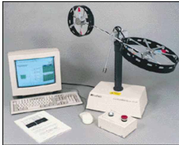
FIGURE 2 TWIN ROTOR PLANT AT CUAS
