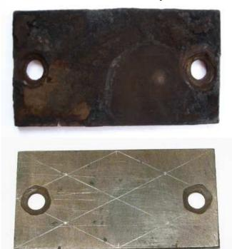
FIG.2 PLOTO OF A CONTROL PLATE. AS IT WAS REMOVED FROM A BOILER (TOP) AND AFTER CLEANING (DOWN). ON THE BOTTOM PLATE VISIBLE LINES WHICH INDICATE MEASURING POINTS. REAL SIZE 100X50 MM [1]
