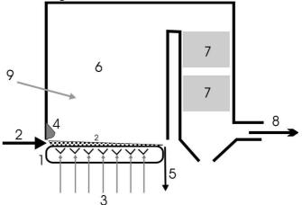
FIG.3 SCHEME OF STOKER BOILER. 1-STOKER, 2-FUEL, 3-PRIMARY AIR, 4-IGNITION WALL, 5-SLAG, 6-COMBUSTION CHAMBER, 7-HEAT EXCHANGERS, 8-FLUE GASES EXIT, 9-SECONDARY AIR
