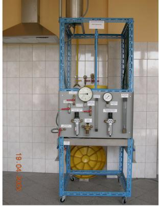
FIG.4 PHOTO OF THE TEST STAND FOR TESTING ATOMIZERS [3] "Hot" tests were done in order to check performance of the designed burner while burning mixture of fuel oil with raw rapeseed. It was found that burner can be fuelled with mixture containing up to 50% of raw rapeseed oil. This project finished in 2005. The effect of student participation is that they learned by-doing how to design atomizer and had opportunity to see the effect of the design process.
