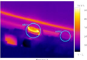
FIGURE 1 THERMAL IMAGE OF BEARING
