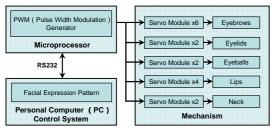
Figure 2 Architecture of an Affective Robot
