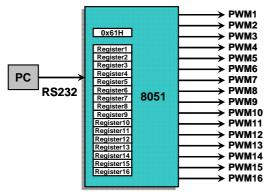
Figure 4. Architecture of the Micro Controller
