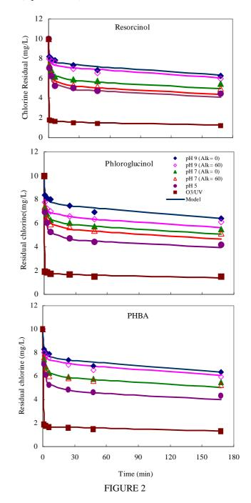
THE MEASURED RESIDUAL CHLORINE CONCENTRATION FOR RESORCINOL, PHLOROGLUCINOL, AND *P*-HYDROXYBENZOIC ACID AT VARIOUS REACTION TIMES
