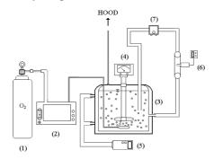
(1) Oxygen cylinder; (2) Ozone generator; (3) Batch reactor;
