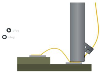
FIGURE 2 Ultrasonic wire bonding (frame B)
