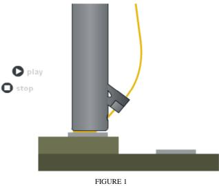
ULTRASONIC WIRE BONDING (FRAME A)
