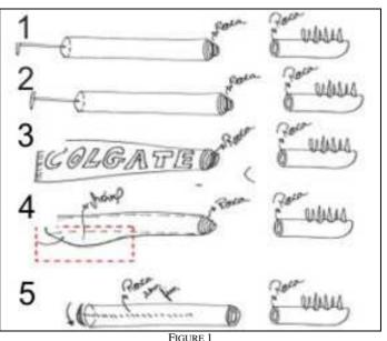
TOOTHBRUSH STUDIES WITH THE DIVERSE ALTERNATIVES GENERATED. 1)FIXED PISTON, 2)MOVABLE PISTON, 3)ADAPTED HEAD, 4)FLEXIBLE HANDLER AND 5)ENDLESS THREAD
