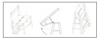
FIGURE 2 BASIC CONCEPT OF THE "STAIR CHAIR" DESIGN
