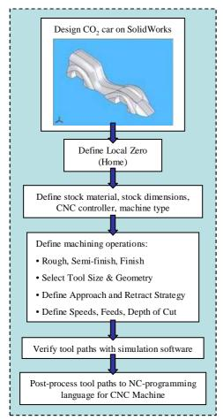
FIGURE 4 SOFTWARE TASKS WITHIN THE CAM MODULE
