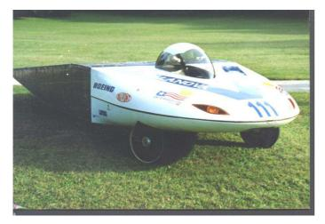
FIGURE 1 PHOTOGRAPH OF SOLAR CAR DESIGNED AND BUILT BY VILLANOVA UNIVERSITY STUDENTS
