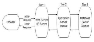
FIGURE 7 THREE TIERS OF X3D SIMULATION WEB
