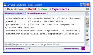
FIGURE 4 DEFINITION OF EXPERIMENT I IN EJS.
