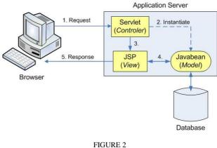
SYSTEM'S SOFTWARE ARCHITECTURE (MVC ARCHITECTURE)
