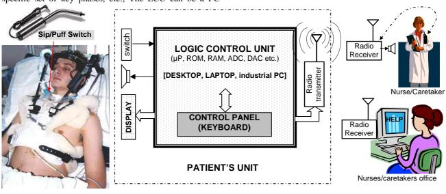
FIGURE 1 The hardware structure of the system
