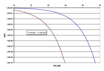
FIGURE 1 BIT ERROR RATIO VS. SIGNAL-TO-NOISE FOR SEVERAL LEVELS OF M-QAM
