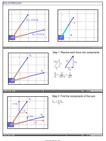
FIGURE II WALKTHROUGH EXPLAINING THE ADDITION OF FORCES BY COMPONENTS.
