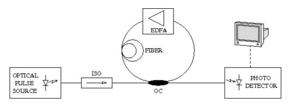
FIGURE 2 LABORATORY SET FOR LONG-HAUL OPTICAL TRANSMISSION SIMULATION. ISO – OPTICAL ISOLATOR, OC – OPTICAL COUPLER, EDFA – ERBIUM-DOPED FIBER AMPLIFIER
