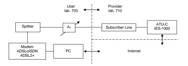
FIGURE 1 LABORATORY SET FOR ADSL MEASUREMENT. ATTENUATION ELEMENT (A1).
