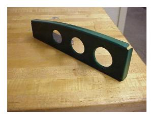
FIGURE 4 FORMED WING RIB.
