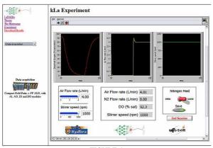
FIGURE 4 MAIN SCREEN OF THE GASSING OUT METHOD.
