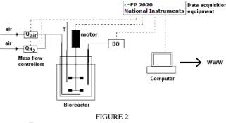
EXPERIMENTAL SETUP USED FOR KLA DETERMINATION.
