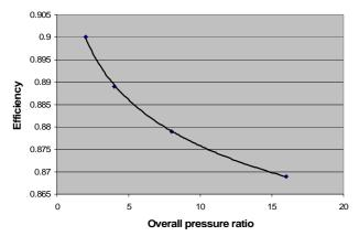
FIGURE 3 Overall Compressor Efficiency vs. Pressure Ratio
