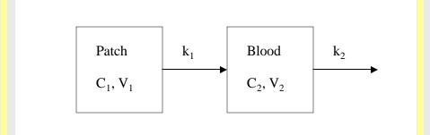
$$\frac{dC_1}{dt} = \frac{-k_1C_1}{V_1}$$
