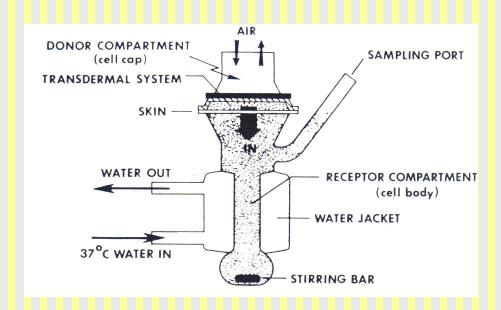
Apparatus used to perform *in vitro* experiments to determine the flux of a drug through skin, from Kydonieus, A. F. and B. Berner, *Transdermal Delivery of Drugs*, Volume II (Boca Raton, FL:CRC Press, 1987).
