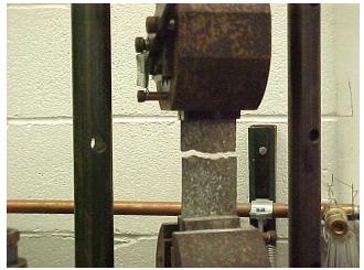
• The simulated lap joints were cut in 1.5 wide pieces and tested to destruction in a tensile tester to determine how much strength was lost due to corrosion damage.
