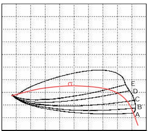
A typical impedance plane display representing the thicknesses at the 5 locations on the thinning standard
