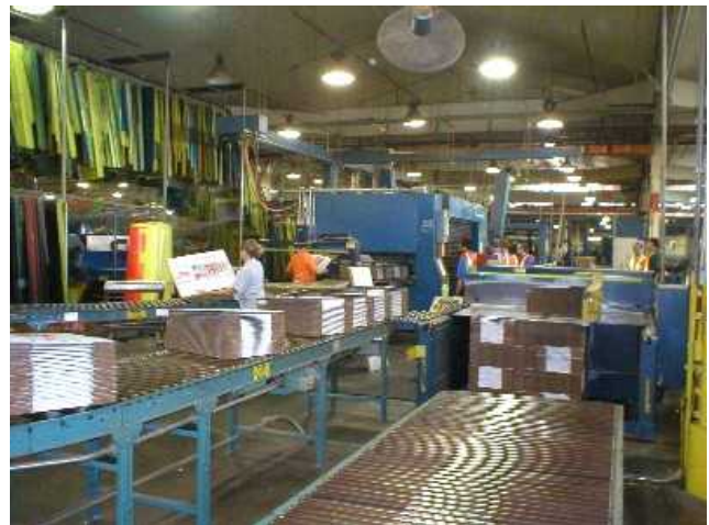
FIGURE 2. A few vies of part of the process shown to the class as a case study of a cardboard boxes manufacturing facility in the US. The Corrugator is shown on the left, and the Flexo machine with the final product are shown on the right.
