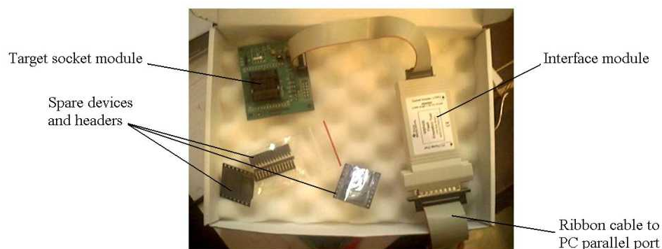
FIGURE 1 THE MSP430 FLASH EMULATION TOOL.
