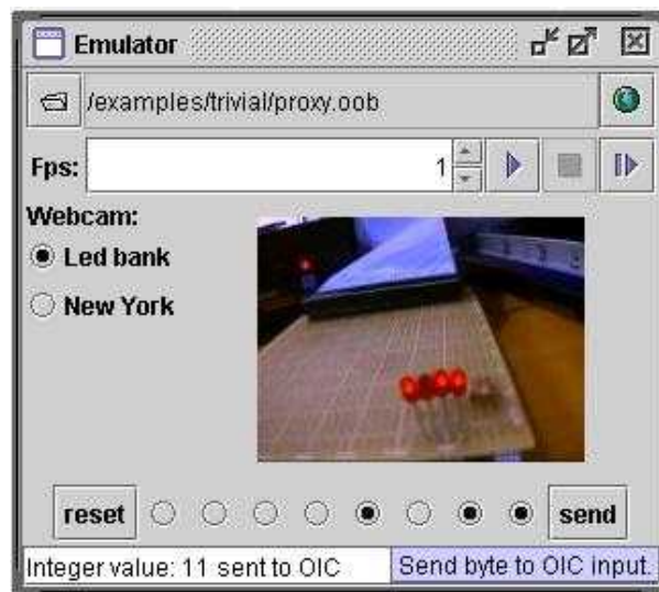
FIGURE. 3 EMULATOR PROGRAM . FOUR LIGHT EMITTING DIODES CONNECTED TO THE OIC PROCESSOR
