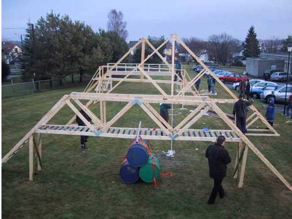
FIGURE 4 TESTING STRENGTH ON BRIDGE PROTOTYPES.
