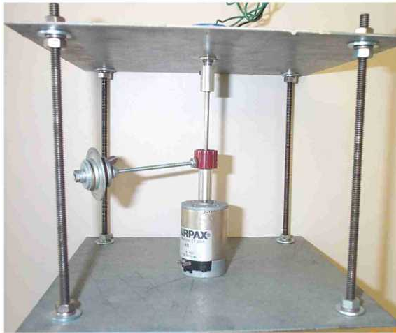
Figure 3: Single link robot mechanical system with top support plate
