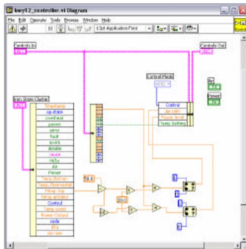
Figure 7 – LabVIEW diagram to implement typical student controller
