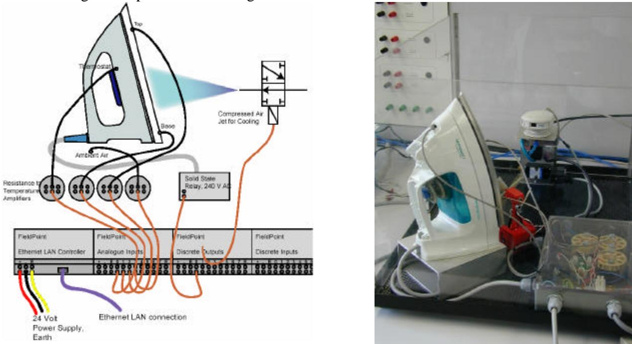
Figure 3a, 3b – Domestic electric iron used for remote laboratory exercises
