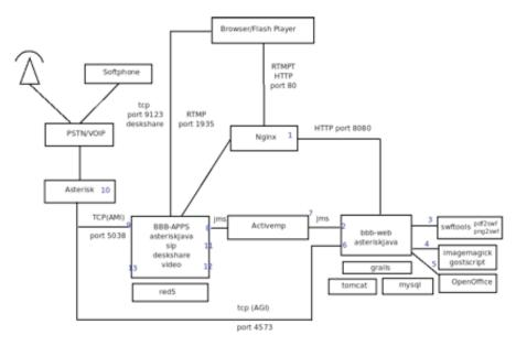
FIGURE 2. Architecture of BigBlueButton [10].
