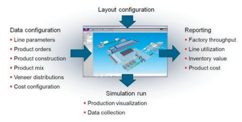
FIGURE 1. Raute's mill simulation concept.
