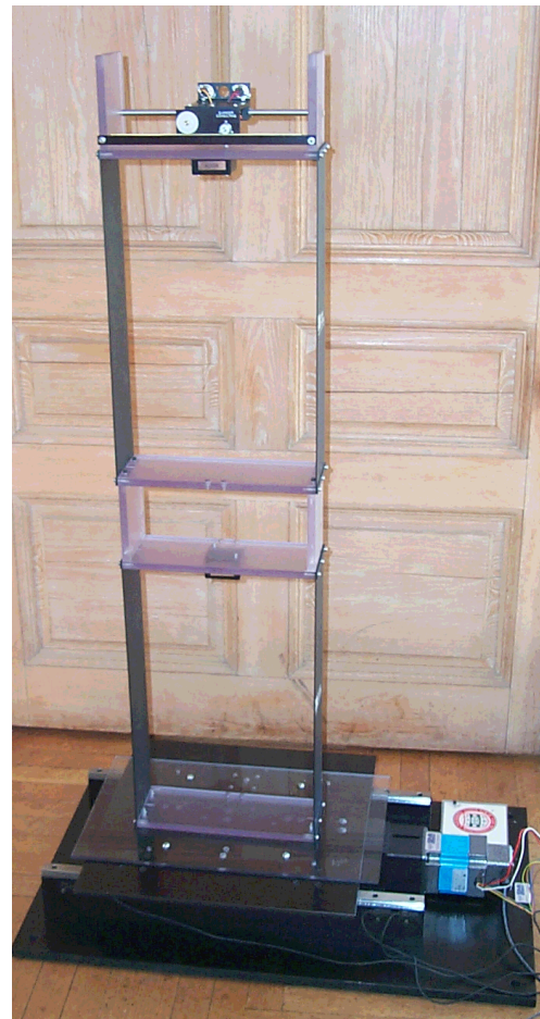
Figure 0 Shake Table Experiment.
