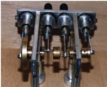
(B) \alpha CONFIGURATION FOUR CYLINDER/ONE CRANKSHAFT HORIZONTAL STIRLING ENGINE MADE BY C.M. WAN (1999).
