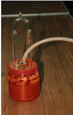
(A) A STIRLING FLUIDYNE PUMP MADE BY F.L. LIAO (1996) (THIS PUMP IS DESIGNED BY A.E.R.E. HARWELL [2].)
