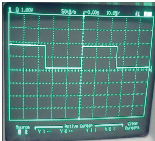
FIGURE 2. LED Voltage Waveform.
