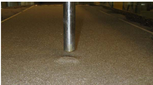
Figure 7. Image of score dune and hole. Cylinder is D/2 above the channel bottom.
