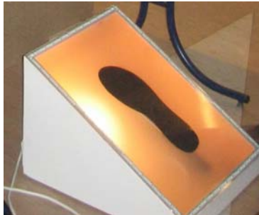
Fig. 1. Prototype of metal detector. Place your shoe on the black field, and if there are any metal in it, the alarm sounds.
