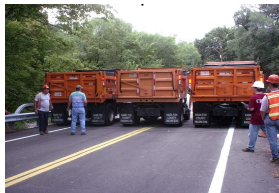
FIGURE 2 TRUCK ON THE BRIDGE DECK FOR TESTING
