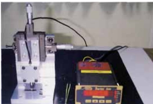
FIGURE 15 SETUP FOR THE LVDT CALIBRATION BY USING GAGE BLOCKS
